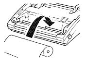
◀ If there is an adhesive sticker sealing the paper roll, remove it completely. Be sure the paper exits from the top of the roll as shown.
